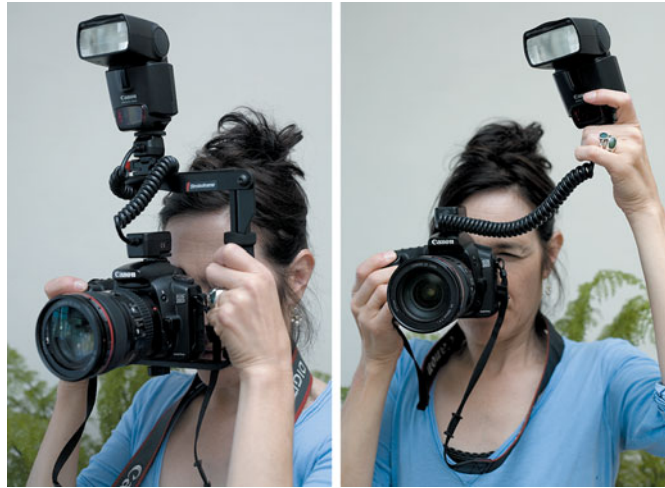
FIGURE 9.13 Off-camera flash brackets allow you to get your flash away from your camera and into a position that will allow you to reduce annoying shadows behind your subject. If you don't have a bracket, you can use an off-camera cable, and simply hold the flash in a better position. (Note that, to use a flash bracket, you must have an off-camera flash cable.)
